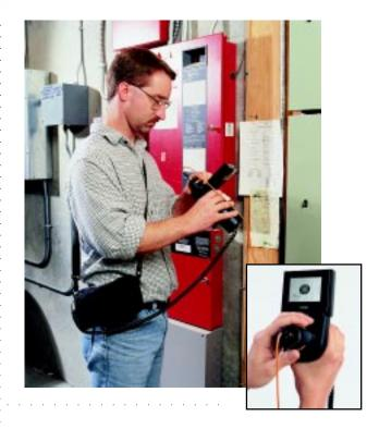
Every year, demands on bandwidth increase. High bandwidth requires cleanliness. The Westover FVPW ensures you can accurately inspect terminations and reduce attenuation. Using the clear LCD screen, debris, contamination, scratches, and core damage is readily identified. Since it is a video system, it is ideal for training and/or group discussions.
