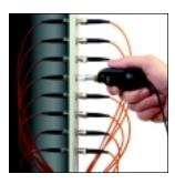
The probe tip mates with the female bulkhead adapter or mating adapter. A variety of dedicated adapters are available which allow you to inspect several types of connectors.
