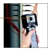
The image of the fiber will appear centered and in sharp detail on the hand held display.
